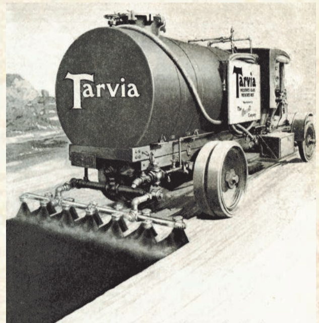
Some poorer counties on the Dixie Highway connectors could only afford to spray tar on a graded dirt road.
